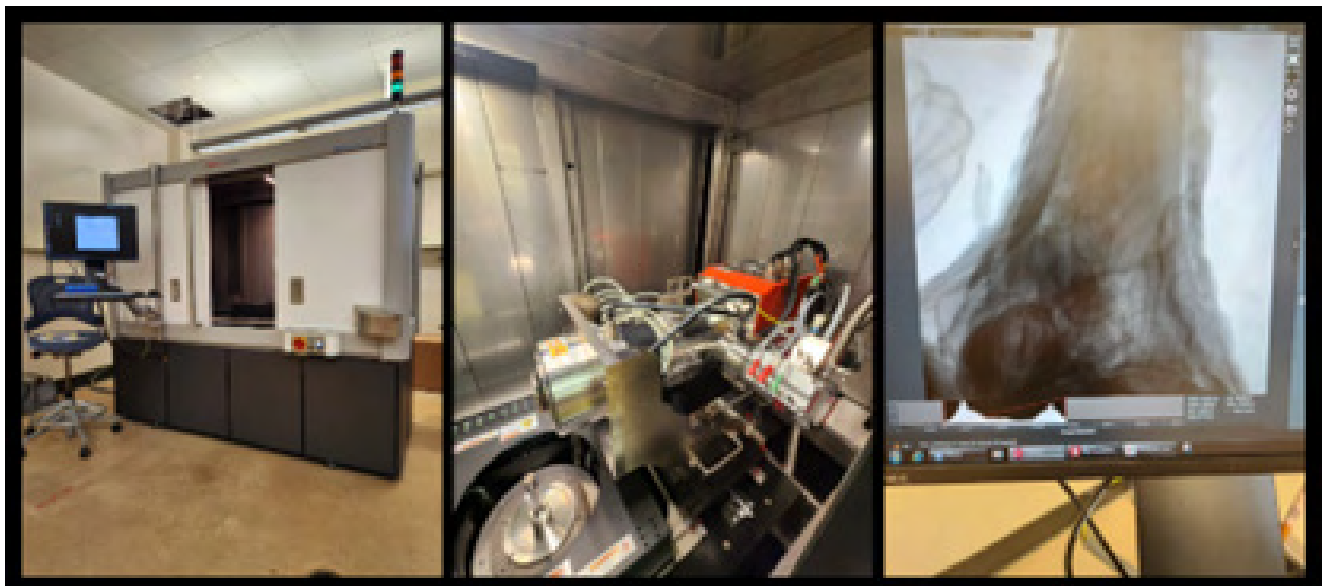
Fig. 3: LSU’s ThermoFisher HeliScan MKII X-ray microscope.
