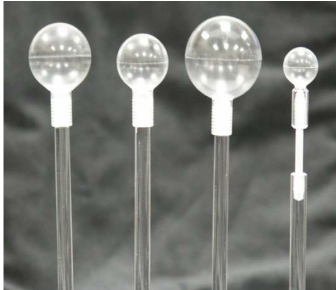
Figure 7: Hot Sphere phantom comprising hollow sphere set.
