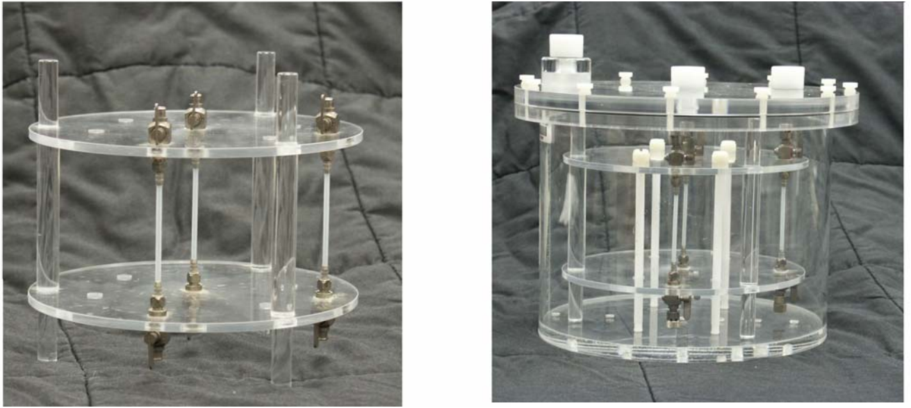
Figure 6: (a) Triple-line phantom and (b) Triple-line phantom mounted inside the ECT cylinder.
