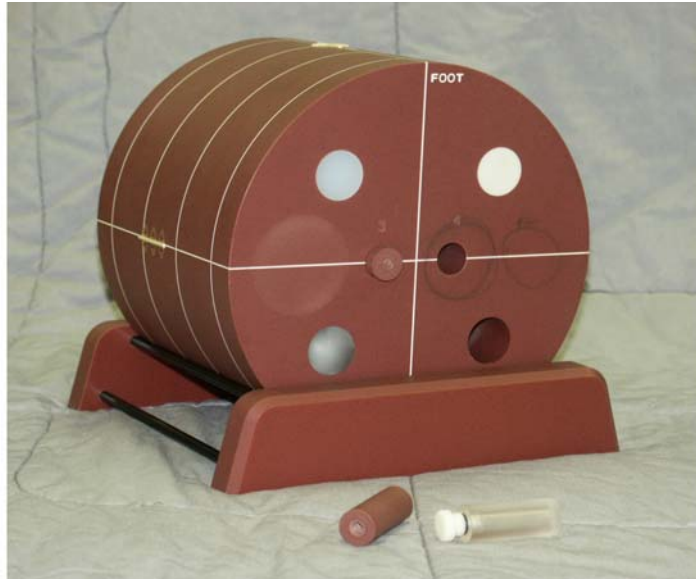
Figure 5: Photograph of the modified Gammex phantom, showing the location of insert holes and the inserts used for this research. Also, the four materials of different densities (bone, acrylic, polyethylene and air) in module 1 of the Gammex phantom can be seen, as can the acrylic and solid water inserts used for holding the radioactive isotopes.
