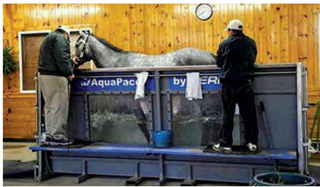
Underwater treadmill by Aqua Pacer allows for adjustment of the water level and water temperature to help rehabilitate horses after injury. https://www.hudsonaquatic.com/products/equine/
